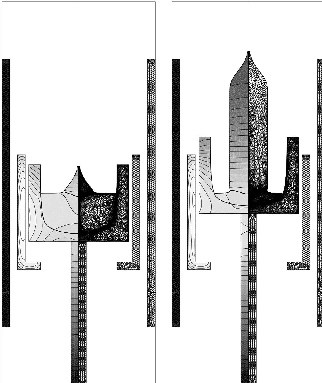
Figure 1. Growth of a 100 mm Si crystal (pulling rate: 0.5 mm/min; crystal rotation rate: 10 rpm; crucible rotation rate: -5 rpm). Temperature field by steps of 50 K and deforming mesh calculated at 2 growth stages by means of a transient FEMAG-CZ.2 simulation.
