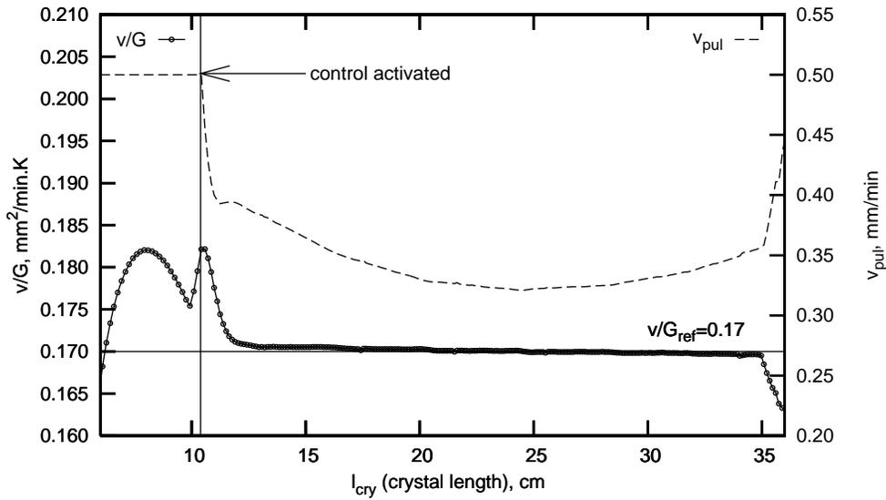
Figure 4. Second transient simulation, with an off-line controlled  $v/G$  ratio while the pulling rate  $v_{pul}$  is the control variable.
