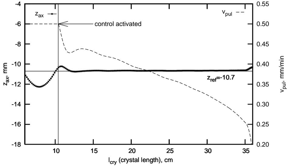
Figure 3. First transient simulation, with an off-line controlled axial interface deflection  $z_{ax}$  while the pulling rate  $v_{pul}$  is the control variable.
