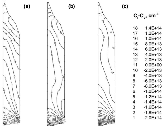
Figure 5. Isovalues of  $C_I - C_V$  in the crystal for the three considered transient simulations of the problem of Fig. 1. (a) uncontrolled simulation; (b) off-line controlled axial interface deflection  $z_{ax}$ ; (c) off-line controlled  $v/G$  ratio.
