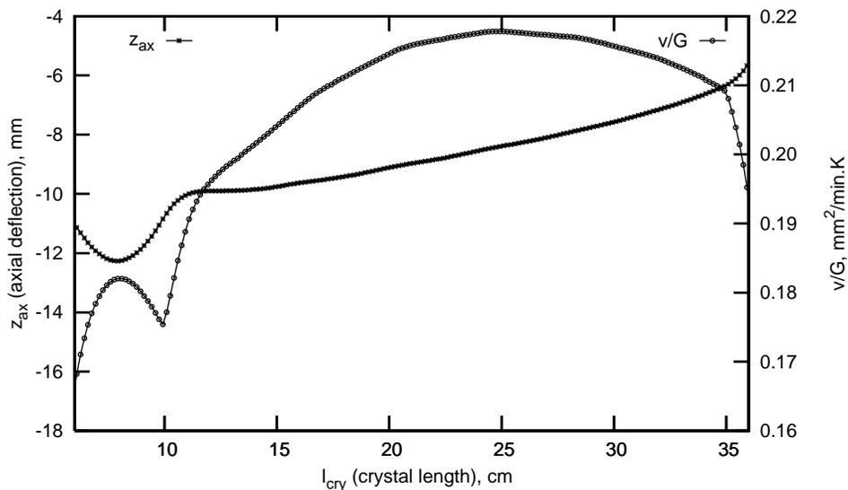
Figure 2. Uncontrolled simulation of the problem of Fig. 1. Evolution of the axial interface deflection  $z_{ax}$  and the  $v/G$  ratio as a function of the grown crystal length  $l_{cry}$ .
